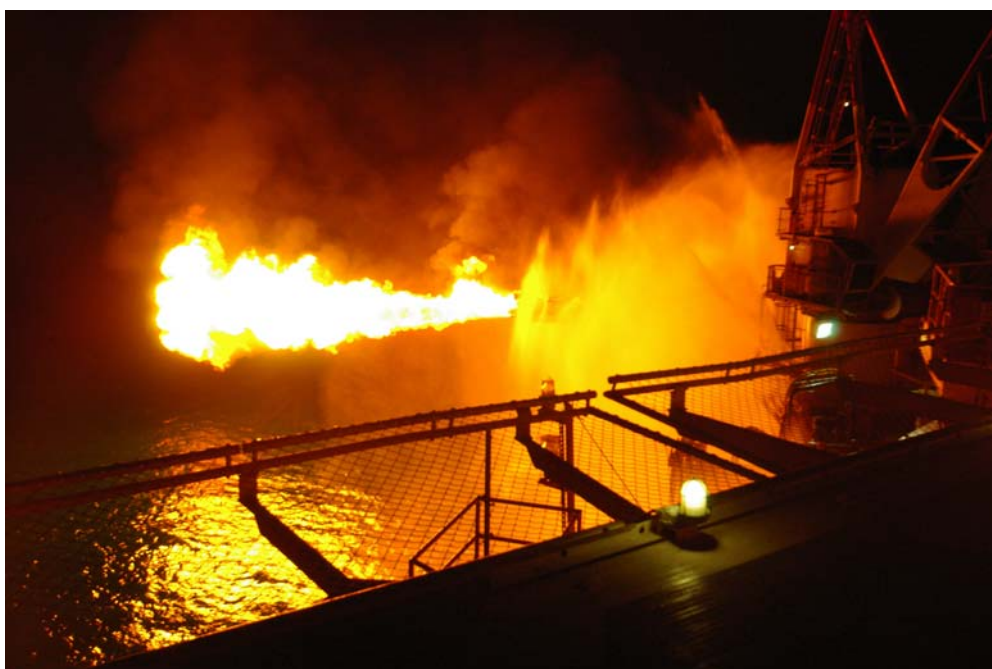
Gas flaring during Longtom -3, test 2 at an estimated flow rate of 59 MMscf/d
