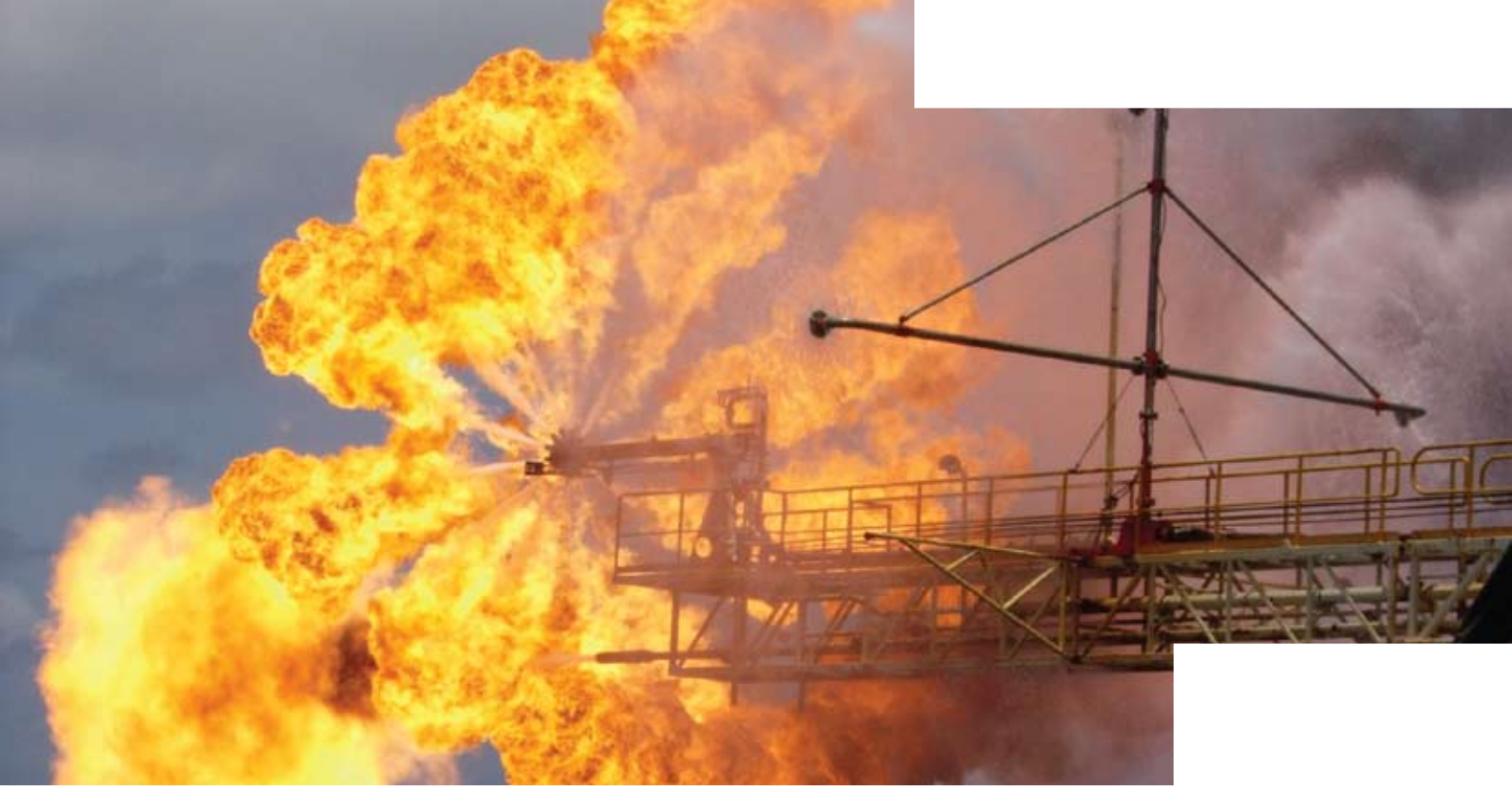
CruX-3 production test flare
